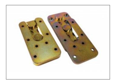
The ATFN is a two piece steel plate connector. The first part of the connector is fixed into a pocket on the header timber with nails and the second part is fitted on the end of the in-coming beam with screws. No slots or dowel holes are necessary, speeding up installation.
