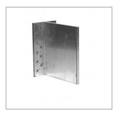
The BTALU concealed hanger is one solution to connecting timber members together without seeing the connector. It is designed to be fixed to the header timber and then fully inserted into a slot in the in-coming beam, and held in place with dowels. Holes are drilled through the timber and fin of the BTALU, allowing accurate alignment. This method provides an aesthectically pleasing connection for feature beams.
