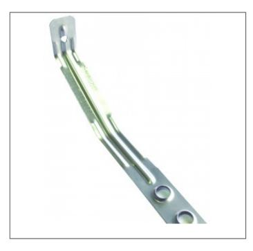
The BTS and SWT wall ties are used to restrain external brickwork back to timber frame building structures. The BTS and SWT offer an outstanding combination of performance and cost in a wall tie for use with timber frame or SIP (Structural Insulated Panels). Allows up to 24mm of differential movement.
