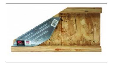
The JES is a two piece metalwork system which enables the use of engineered timber I-joists in loft conversions, offering a safe and economic alternative to the traditional method which requires steel girders. It provides reinforcement to the joist ends where they are cut to fit within the eaves of the existing roof. Each JES is supplied as 2 plates, as required for each joist end.
