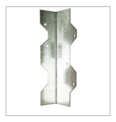
A reinforcing angle designed to transfer loads between 2 ply floor joists/metal web joists. The L70 Reinforcing Angle may be used in pairs to transfer the loads between floor joist plys.
