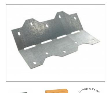
Designed to attach timber members at irregular angles, these connectors can be bent on site from 0° to 135°. The staggered nail pattern reduces the possibility for splitting the timber and allows installation on both sides of the member.
