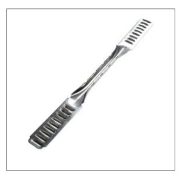
Improve the effective thickness of a wall under load. Maintain the moisture break and thermal/sound insulation characteristics of cavity walls. Designed, manufactured and tested to the BS requirements of DD140 parts 1 and 2. **LWTS: Type 3 Cavity Ties:** General purpose ties suitable for cavity widths up to 75mm. Suitable for use in masonry cavity walls of domestic houses and small commercial buildings up to 15m in height, where the basic wind speed does not exceed 44m/s.
