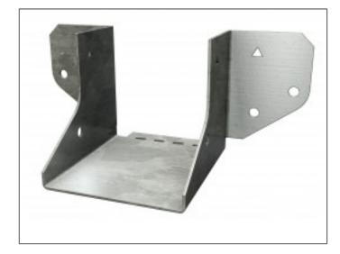
The MH is a one piece galvanised hanger available in a range of widths for light duty applications such as trimmers and ceiling joists of rectangular section. THe MH can also be used to build decking platforms.
