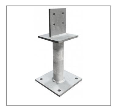
The PBH is suitable for heavy duty post support applications including Glulam timber posts,with a standoff height of 216mm. Dowels included. PBH75 suitable for posts 75 x 75mm to 120 x 120mm PBH120 suitable for posts 120 x 120mm to 200 x 200mm
