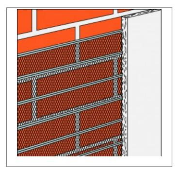
The RBL Bib Lath provides plaster/render backing and is also suitable for the refurbishing of damaged or deteriorated faces of masonry walls. Available in galvanised for internal use and stainless steel for external use.
