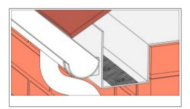
A 75mm wide, fine stainless steel mesh on a 30m roll. Easy to cut and install. Allows roof space ventilation and helps prevent birds and insects from gaining access via soffits.
