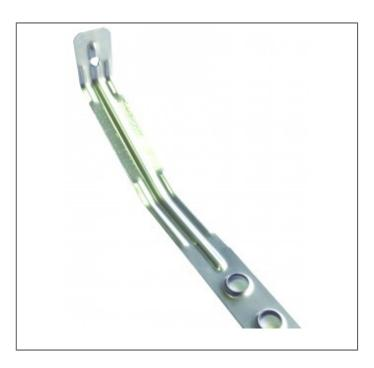
The SWT wall ties are used to restrain external brickwork back to timber frame building structures. The BSWT offers an outstanding combination of performance and cost in a wall tie for use with timber frame or SIP (Structural Insulated Panels). Allows up to 24mm of differential movement.
