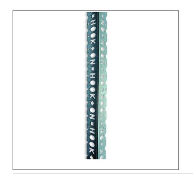
TTCB is pre-toothed thin coat bead that needs no nails or screws, just push and tap it on to the corner of the wall and get plastering. TTCB (toothed thin coat bead), features tiny teeth spaced at 40mm intervals which grip the plaster board, holding the bead firmly in place. Easy to install, just push and tap into place for a firm fit to the plaster board...
