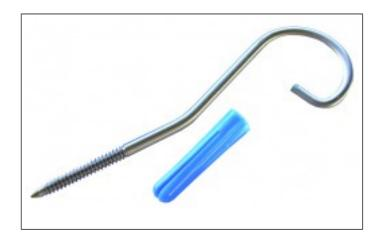
Screw in wall starter with nylon wall plug, WST provides lateral stability to brickwork or blockwork walls. Can be installed horizontally or at a 30° angle to the mortar joint.
