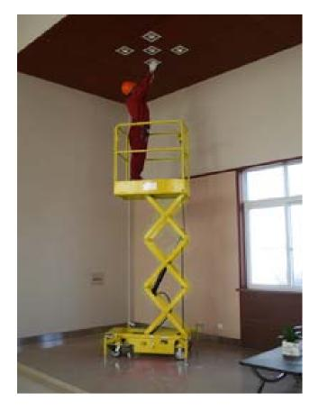
The unit is supplied with an integrated charger, battery charge indicator, built in levelling indicator, outriggers and emergency down and stop buttons.
